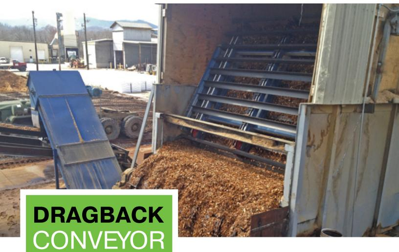
The Drag Back Conveyor from BE&E is the most effective way to make your chain floor bin an accurate feeding device. Live chain conveyors tend to pack material along the top edge of the bin's discharge opening, causing strain on the wall of the bin. Our solution removes all the pressure against the exit wall. In fact, the exit wall can be removed entirely!
